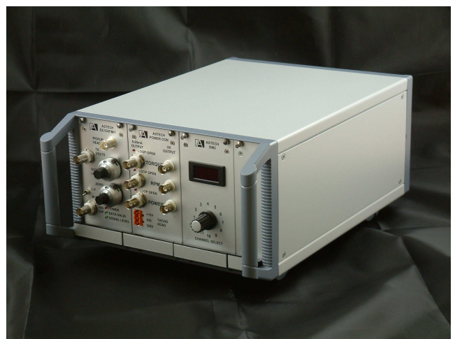
READOUT CASEFRAME CONTAINING DEMODULATOR/DECODER POWER COMPUTATION AND DIGITAL DISPLAY MODULES
