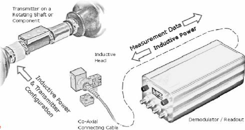
Sensor data collection from rotating or moving components can cause many problems – strain gauge offsets, scaling adjustments, dropouts due to shaft displacements, transmitter power supply difficulties – these are familiar problems to engineers. The new rotary telemetry system from Astech eliminates these difficulties:
