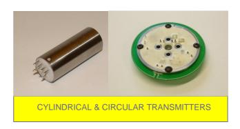
Electrical power for the transmitter is supplied by noncontacting inductive coupling from either a shaft adjacent head or a loop located around the shaft. The transmitter may also be powered by a battery.
